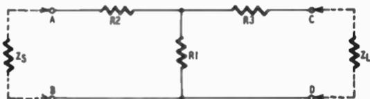
a source impedance  $Z_s$  of 600 ohms to a load impedance  $Z_L$  of 250 ohms. Since we already have decided upon a value for  $k^2$  of 25 db, we do not need to work out equation (13). Using equation (14) to solve for  $k$  we get:
