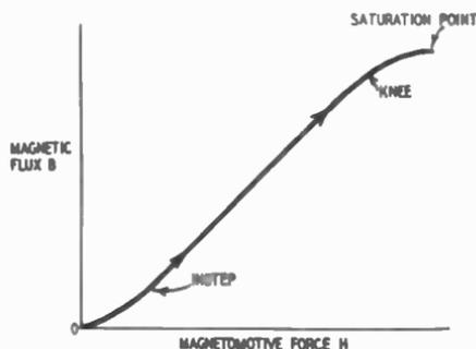
Fig. 921. Normal magnetization curve.
